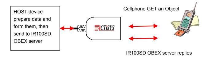
Please note that based on OBEX requirements, when user's host is going to send data to IR100SD-OBEX-Server to response GET command, user's host should tell IR100SD-OBEX-Server how big the object is first. So there is a formatted frame that user's host should obey when it sends this object.
